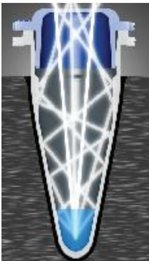
White tube with transparent optical cap High S/N Ratios
