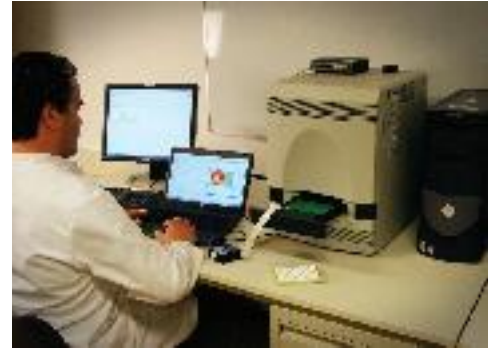
ISO17025 accredited calibration of a qPCR cycler in process. The outcome is validated against defined requirements and is also used to normalize its performance.
