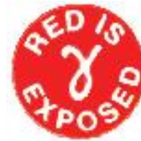
60 Co irradiation exposed sticker as sterility indicator
