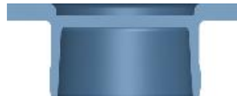
Indented qPCR Cap, the optical area is recessed into the optical cap surface to prevent "touching" the optical area.
