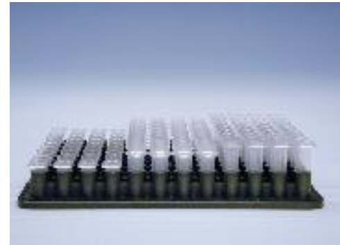
The difference between low, regular and high profile strips
